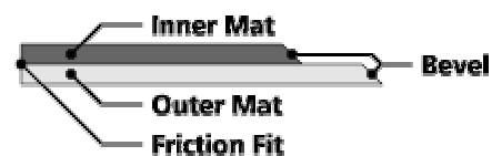
Figure 5. Cross-section of a friction-fit double mat
